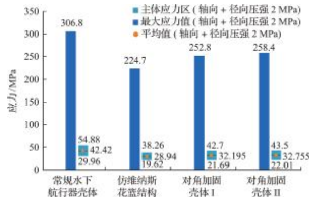
图 13 四种壳体结构施加轴向和径向压强的应力对比 Fig. 13 Stress comparison of axial and radial pressures applied to four shell structures
