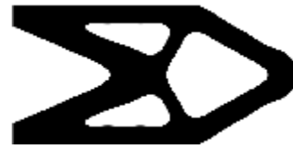
图6 5 Hz下悬臂梁拓扑设计( J=8.99 ) Fig. 6 Topology design of the cantilever beam under 5 Hz ( J=8.99 )
