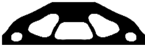
图3 MBB梁拓扑设计( l_c=24\text{ mm} , J=4.38 , DV=111 ) Fig. 3 Topology design of the MBB beam( l_c=24\text{ mm} , J=4.38 , DV=111 )
