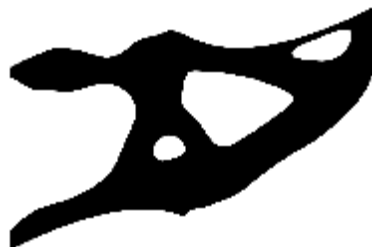
图 16 1000 Hz 下曲形悬臂结构拓扑设计( J=20.34 , J_d=2.03 , J_s=18.31 ) Fig. 16 Topology design of the curved cantilever structure under 1000 Hz ( J=20.34 , J_d=2.03 , J_s=18.31 )
