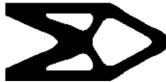
图8 170 Hz下悬臂梁拓扑设计( J=11.49 ) Fig. 8 Topology design of the cantilever beam under 170 Hz ( J=11.49 )
