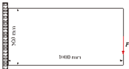
图5 悬臂梁的设计域和边界条件 Fig. 5 Design domain and boundary conditions of the cantilever beam
