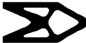
图7 100 Hz下悬臂梁拓扑设计( J=9.79 ) Fig. 7 Topology design of the cantilever beam under 100 Hz ( J=9.79 )
