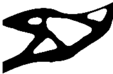
图 15 100 Hz 下曲形悬臂结构拓扑设计( J=17.42 ) Fig. 15 Topology design of the curved cantilever structure under 100 Hz ( J=17.42 )
